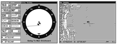
Navigating to Man Overboard: Navigation Page, left, and Map Page, right. The victim is astern of the vessel; the GPS shows which direction to steer to for the rescue.
